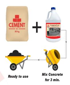
Dosage: 1:3 ratio & Samplus conproof with cement. Quantity many vary depanding on site condition.
